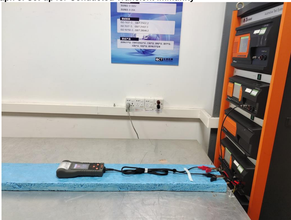
Photograph 3: Set-up for Conducted Transient Immunity
