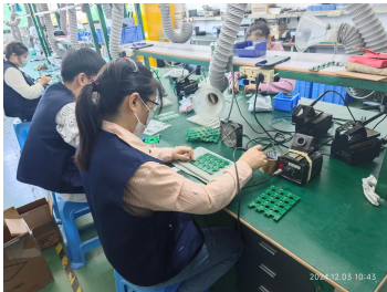
NC-The soldering workers worn activated carbon masks instead of dust masks during work.jpg
