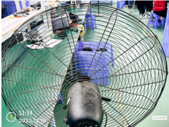
Fans were protected a guard with openings larger than law requirement..JPG
